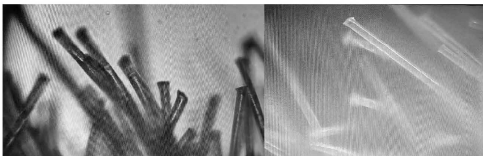
Figure 1 and 2 Nylon hollow fibers at the broken end of test swabs.
